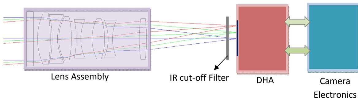
**Fig.3: Schematic of MCC payload**
