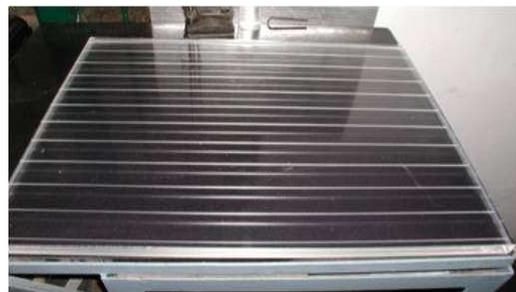
Figure 3(a): Plastic Scintillator used in Experiment.
