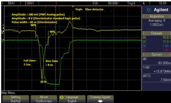
Figure 4(b): Linear pulse characteristics obtained for single fiber detector
