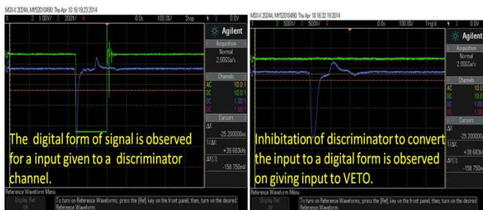
Figure 6: VETO Function in Model 704 Quad four channels Discriminator.
