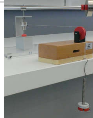
FIG. 2: Rotation apparatus with a weight placed on a weight hanger.
