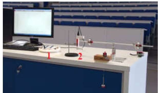
FIG. 3: Rotation apparatus with the system IP – Coach: 1 – CoachLab panel (interface), 2 - optical gate.
