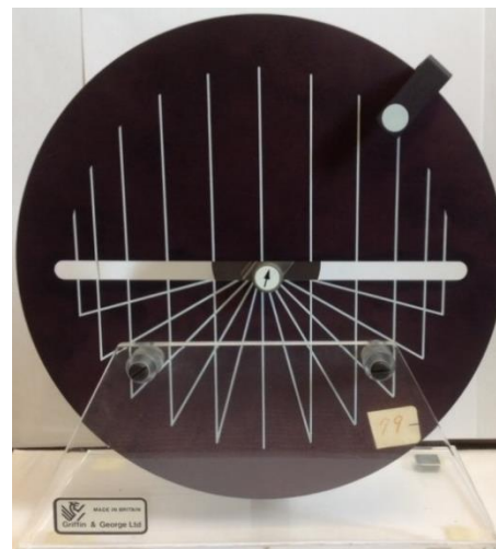
Figure 8. A demonstration equipment illustrating relation between a circular and harmonic motions.
