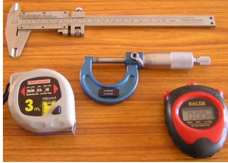
Figure 5. Stopwatch, measuring tape and vernier calipers and micrometer screw gauge
