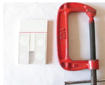
Figure 4. Acrylic support with glass slides fixed on it and the G-clamp
