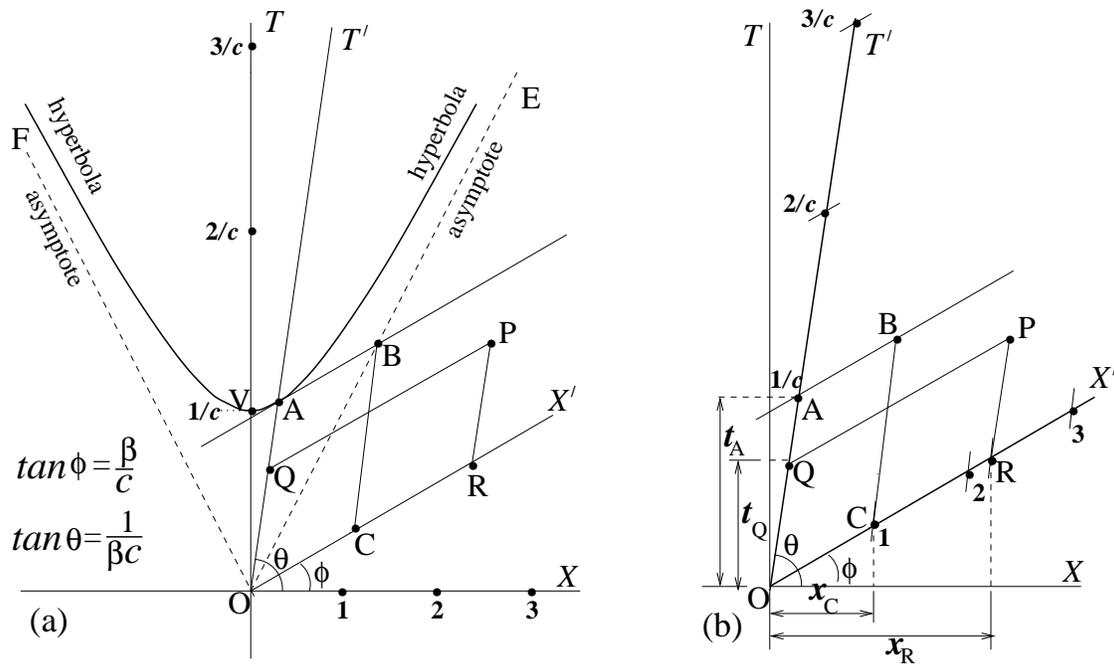
Figure 5: Graphical construction of Lorentz transformation.
