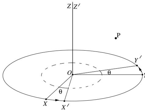
Figure 2: Rotation about the Z axis.
