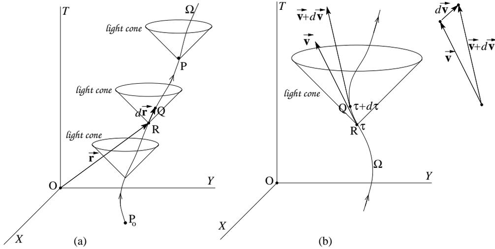
Figure 12: Construction of velocity and acceleration 4-vectors
