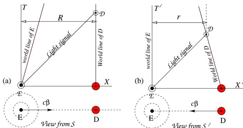
Figure 15: Emission and detection of a light pulse seen from two frames seen in space-time.
