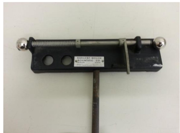
Figure 1. Free-fall and projectile motion demonstration apparatus, shown locked in a “loaded” position.
