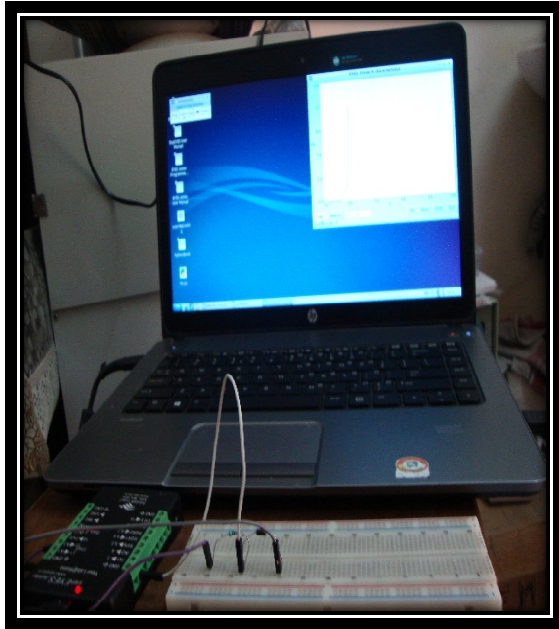
Figure 2. Automated Set-up. The circuit, Expeyes and Data acquisition on the computer
